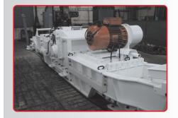
The Coal Crushers DU series was developed for crushing coal, stone or other materials having strength of up to 130 MPa. They are located in entries within the scraper conveyor line. They can be used in connection with different types of scraper conveyors, and with underface equipment.
