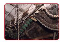
The cable holders in various designs serve for their safe position on the under-working face equipment.
