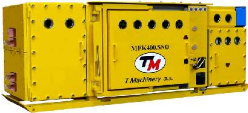
The *Tension Converter MFK 400.SNO* is made of non explosive implementation and is intended for coalmines with classification I M2. The inner parts of the equipment comply with protection level IP 54. The *Tension converter MFK 400.SNO* serves for connecting traverse motor of combine.
